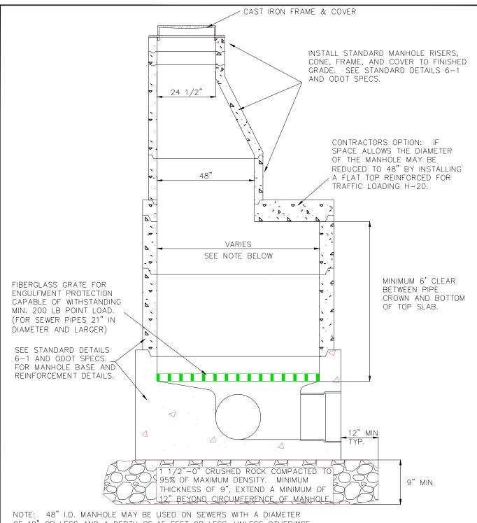
NOTE: 48" I.D. MANHOLE MAY BE USED ON SEWERS WITH A DIAMETER OF 18" OR LESS AND A DEPTH OF 15 FEET OR LESS, UNLESS OTHERWISE DIRECTED BY THE ENGINEER.
