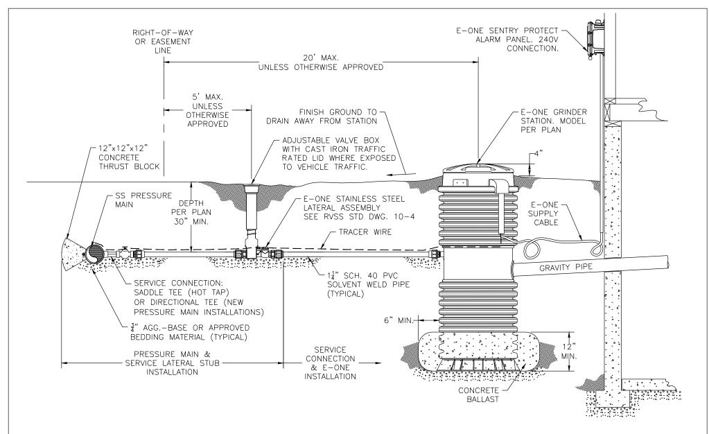
NOTE: INSTALL 14 GAUGE INSULATED COPPER TRACER WIRE FULL LENGTH OF PIPE. LEAVE PUMP END CLEARLY SHOWN AND MARKED INSIDE TANK. WHEN CONNECTING TO EXISTING TRACER WIRE, USE A WATER TIGHT WIRE CONNECTOR OR INSTALL C.O WITH BOTH ENDS OF TRACER WIRE CLEARLY EXPOSED ABOVE FINISHED GRADE.
